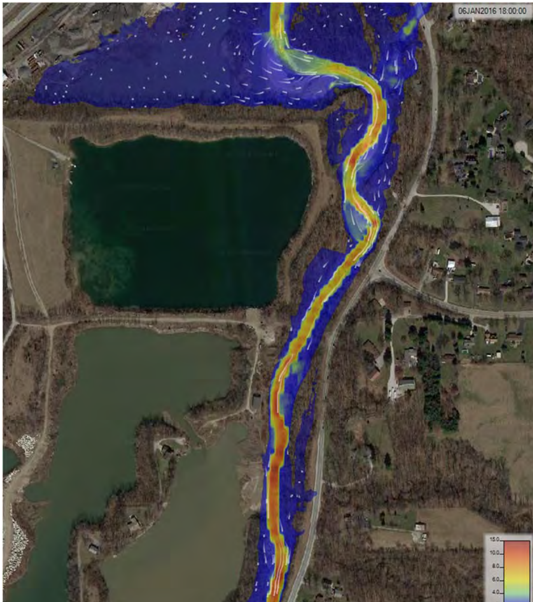
Bankfull Velocity Grid w/flowlines
