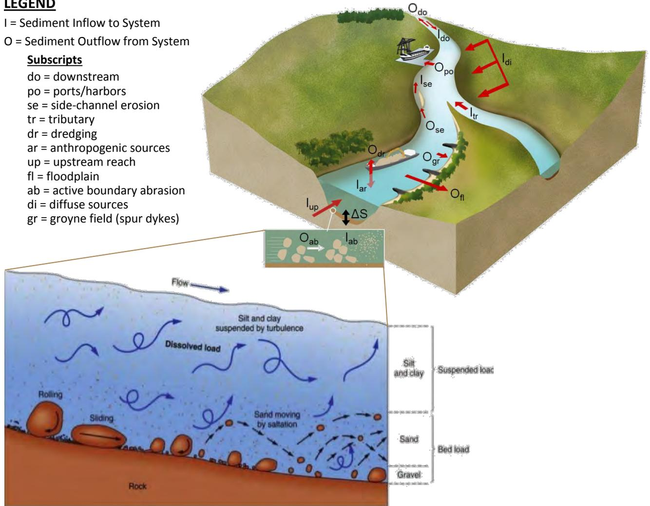
**Figure 4-8: Sediment Transport through a River System**
