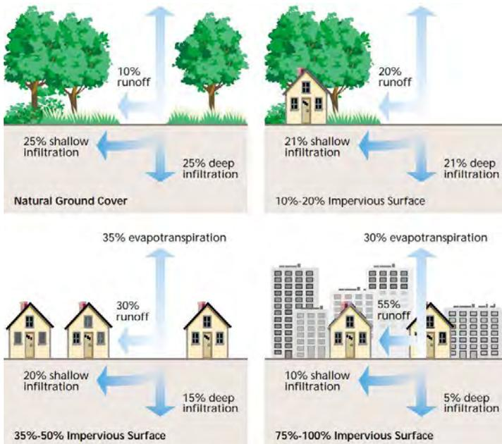
**Figure 4-20: Effects of Urbanization on Runoff**
