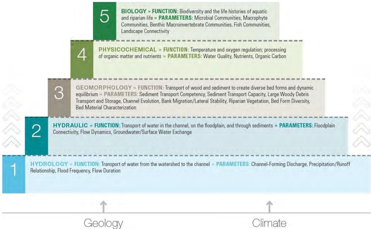
**Figure 3-3: Stream Functions Pyramid**
