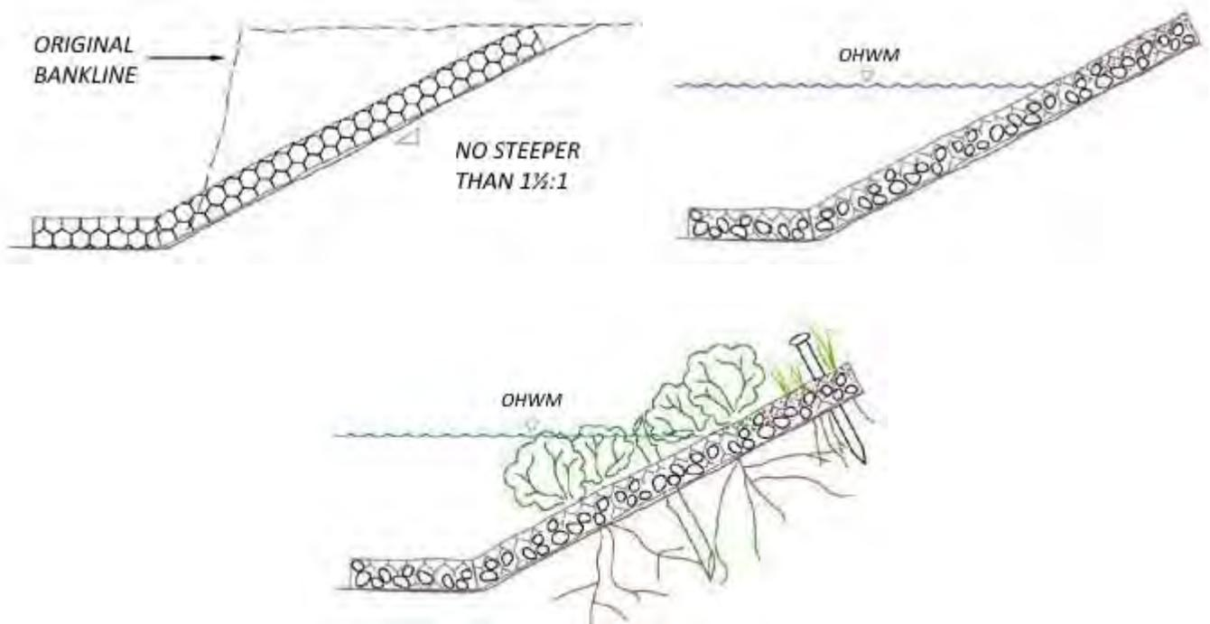
*Gabion mattresses shown in bank installation. Stream bed installation uses the same installation/design techniques to cover and protect the stream bed. Stream bed applications should also extend to just above the OHWM.*
