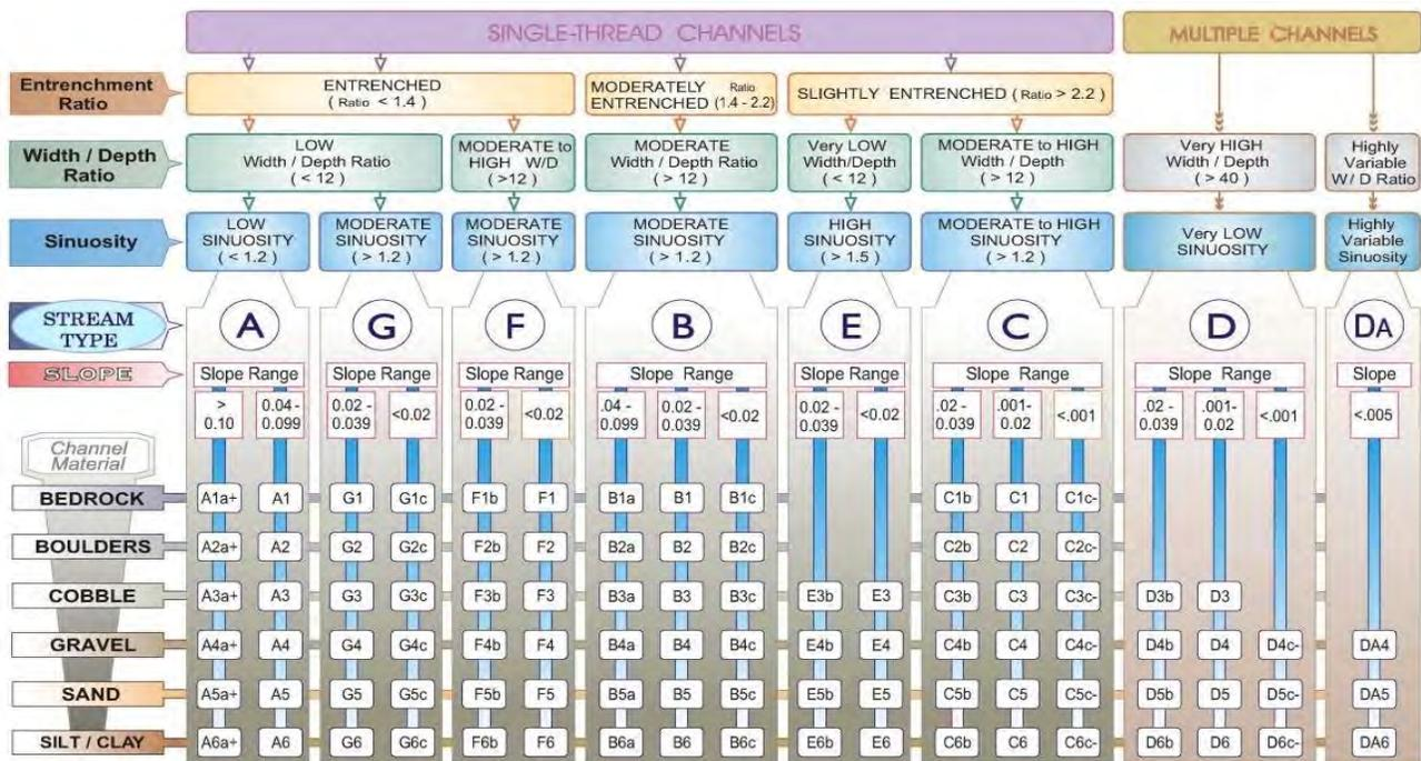
KEY to the **ROSGEN** CLASSIFICATION OF NATURAL RIVERS. As a function of the "continuum of physical variables" within stream reaches, values of **Entrenchment** and **Sinuosity** ratios can vary by +/- 0.2 units; while values for **Width / Depth** ratios can vary by +/- 2.0 units.
