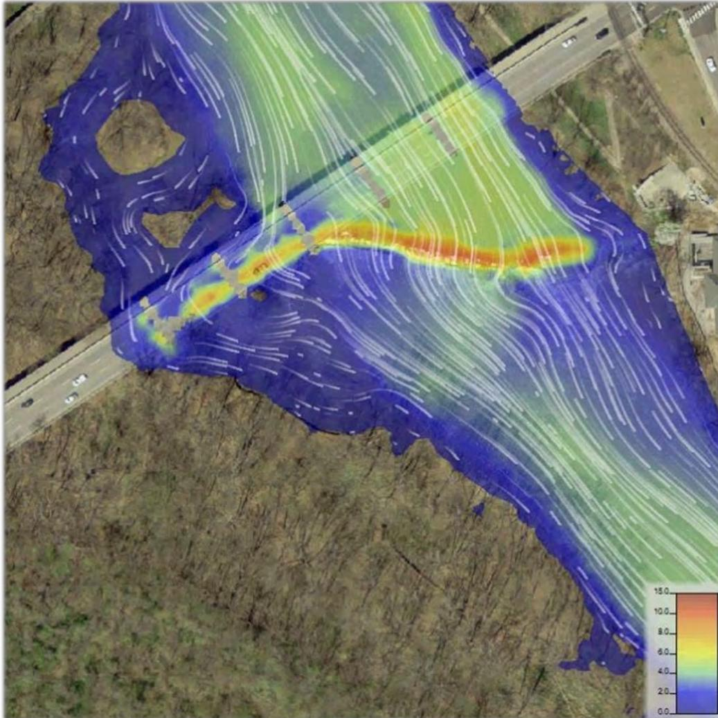
**Figure 3-9: Two-dimensional Model Output for East Fork White River**
