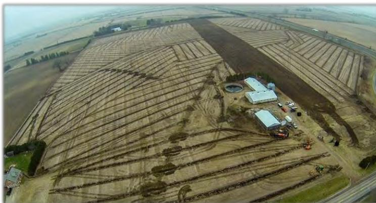
**Figure 4-18: Extensive Tile Drainage**
