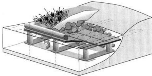
**Figure 4-36: Constructed Habitat – Lunker Structure**
