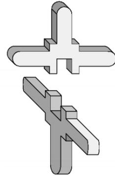
Jacks Formed By Sliding Two Identical Sections Together
