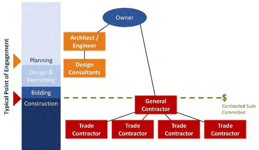
**Figure 4-37: Design-Bid-Build Project Delivery**
