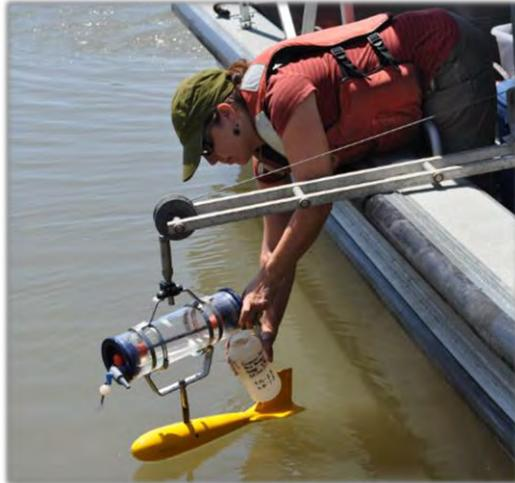
**Figure 3-11: Suspended Sediment Sampling**
