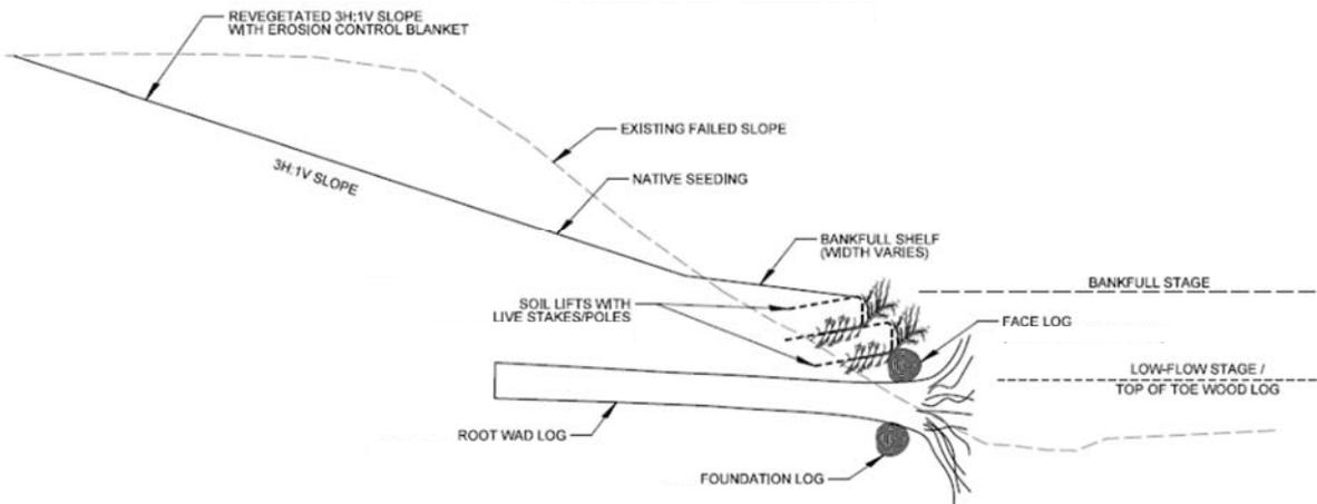
TYPICAL SECTION - TOE WOOD DETAIL
