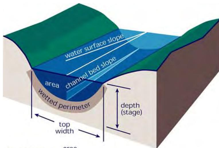
$$\text{mean depth} = \frac{\text{area}}{\text{top width}}$$
