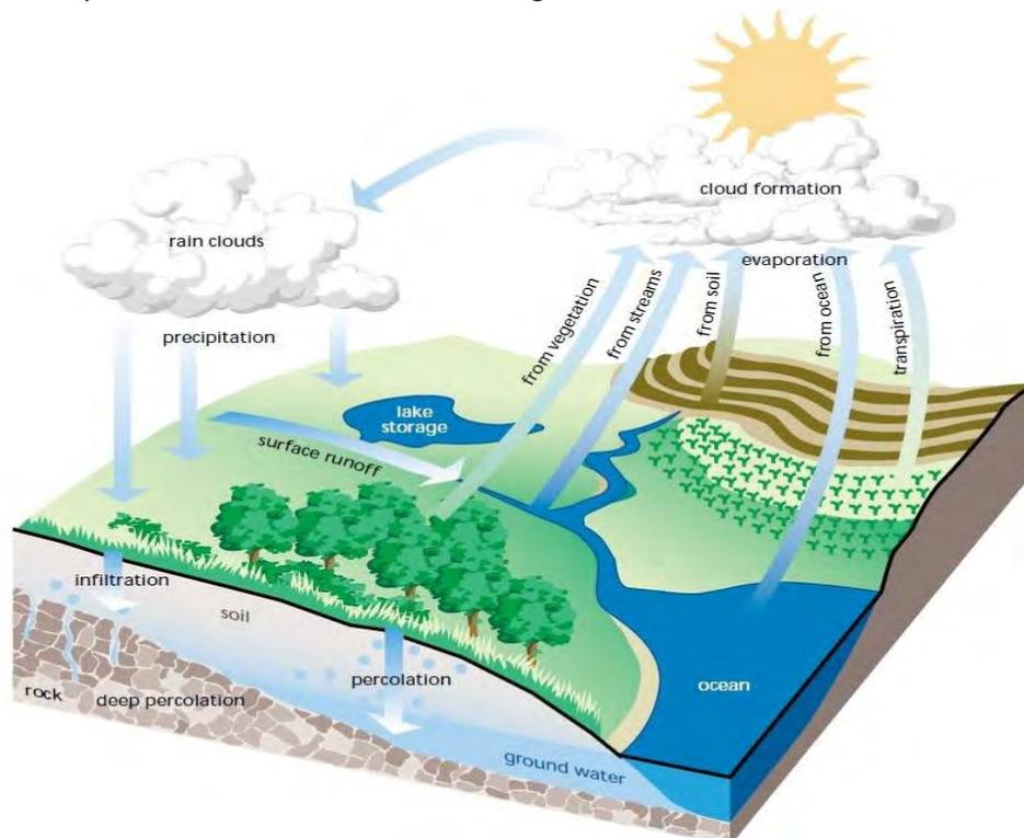
**Figure 3-7: The Hydrologic Cycle**
