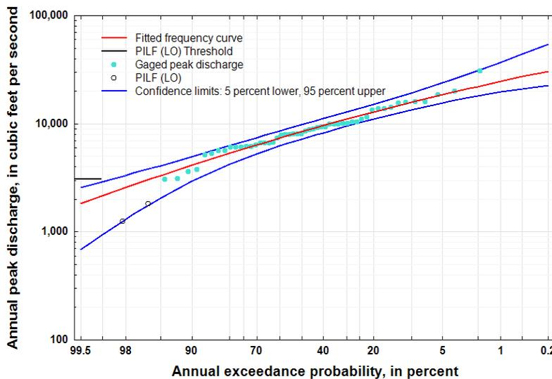
**Figure 4-6: Statistical Analysis of USGS Gage Data using B-17C**
