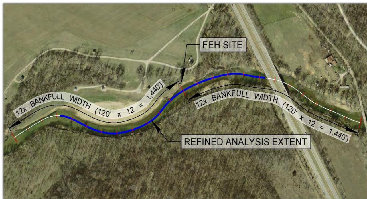
**Figure 4-2: Preliminary Study Reach Limits vs. Refined Analysis Extent**
