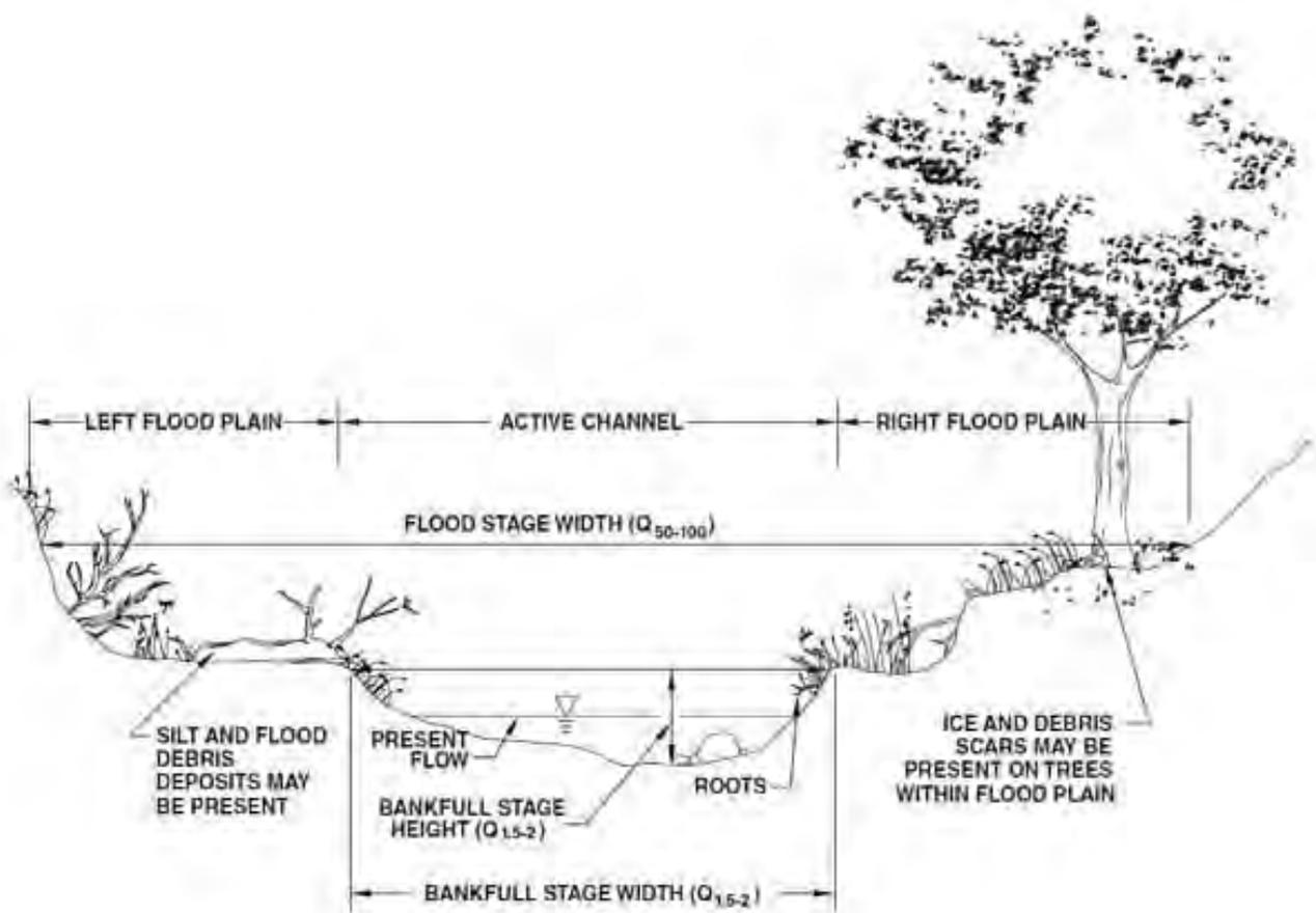
**Figure 4-4: Channel Cross-section with Bankfull Indicators**
