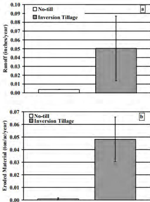
**Figure 4-15: Runoff and Erosion from No-till and Inversion Tillage**
