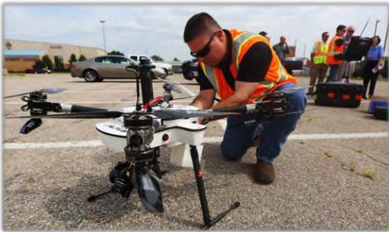
**Figure 5-4: Post-construction Monitoring with Unmanned Aerial Vehicles**
