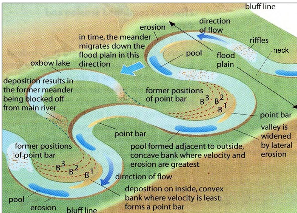
Figure 4-29: Typical Stream Meander Geometry and Progression
