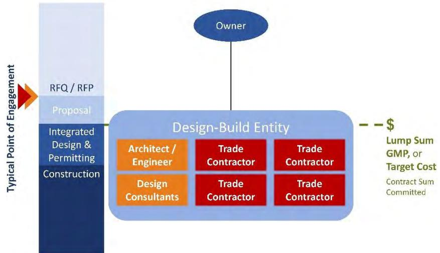
**Figure 4-38: Design-Build Project Delivery**
