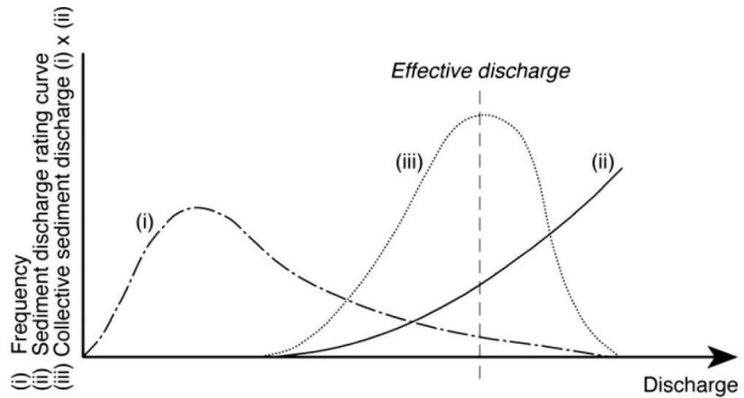
**Figure 4-5: Effective Discharge Determination**
