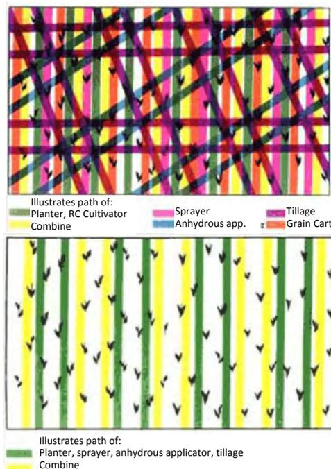
**Figure 4-17: Unmanaged vs. Controlled Equipment Paths**
